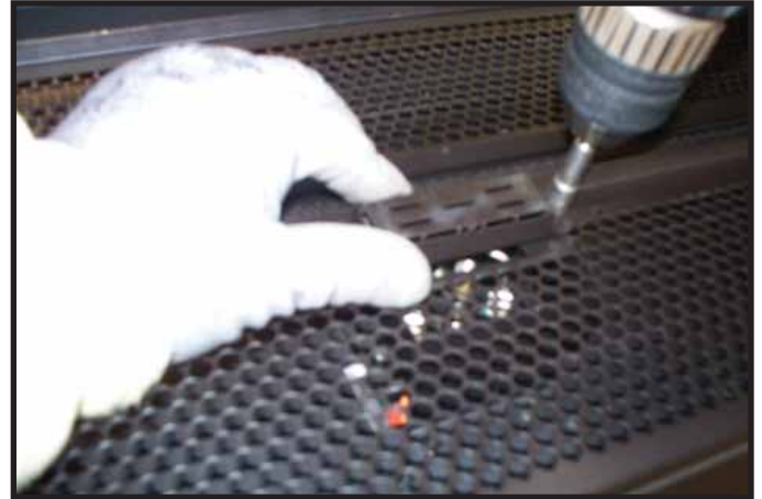
Figure 12.8 Removing Pilot Shield
